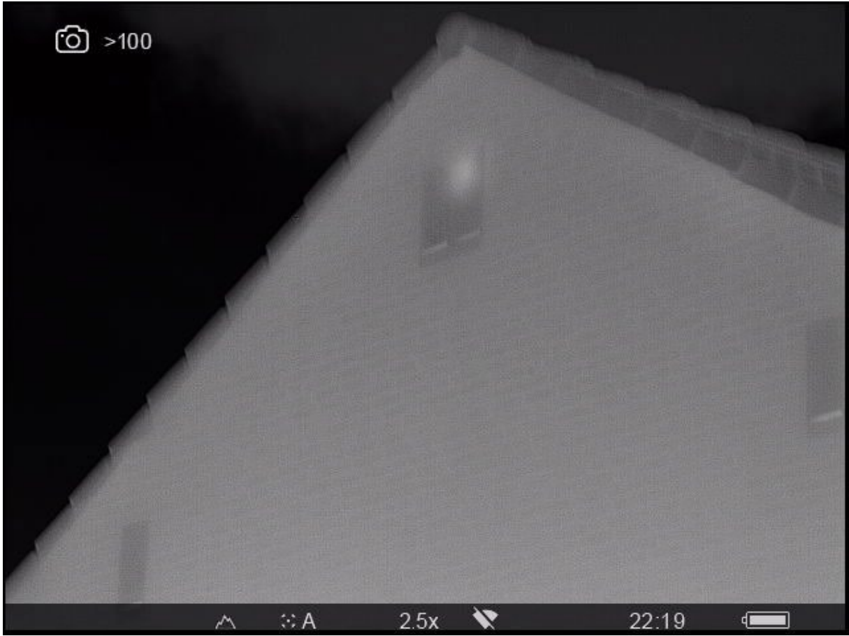
Figure 1: A thermal imaging camera clearly shows the heat from a group of bats in an integrated VMPM bat box. In this case, it was a large maternity colony. Photo: Rick Wortelboer via LinkedIn.
